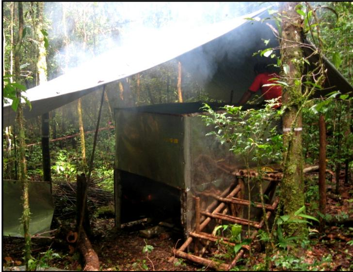
**Fig. 2.** One of the field ovens to dry the subsamples on location.
